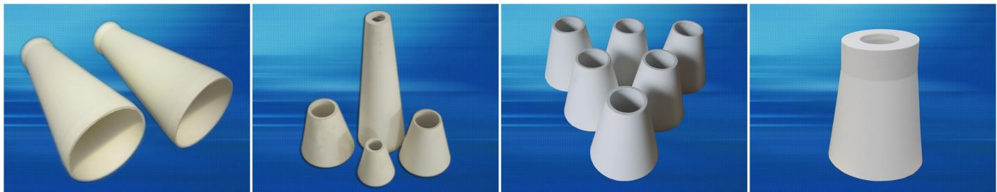
When cyclone is at work, the rotary motion of material generates great centrifugal force, the inwall of cyclone is worn at high speed. For dense material, the abrasion of inner is extremely worse under high impact by centrifugal force. One-piece alumina ceramic tube is used as wear resistant lining in cyclone by its high hardness, strength, abrasion resistance and economic practicality.
